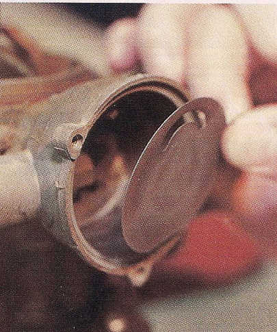
5. With the stat cover and spring assembly removed, the choke baffle plate was removed.
