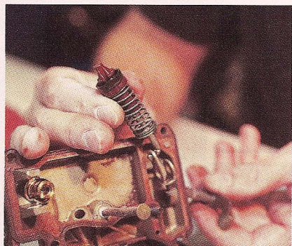
10. A flathead screwdriver was used to loosen then remove the accelerator pump plunger shaft and assembly.
