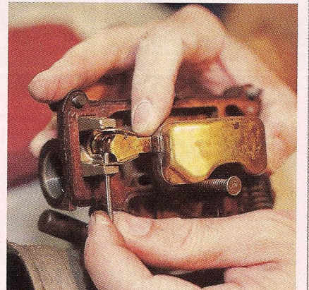
9. Rotating the top half of the carburetor allowed access to the float hinge pin, which was then removed.
