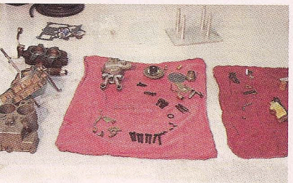
18. After the Rochester 2GC carburetor components and parts were thoroughly cleaned, they were laid out for inventory and inspection.
