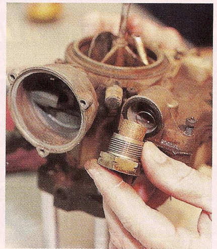
7. To gain access to the fuel filter and spring, the fuel inlet fitting was loosened and removed.
