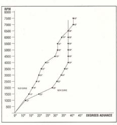
rotating the plate and advancing the timing. Each distributor is recurved according to the specific engine application. By looking at the graph, you can see that the curve of the modified distributor comes in quicker at lower rpm and gradually increases at higher rpm.
