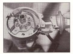
With the stock timing advance figures plotted, Murphy disassembled the distributor for recurving by removing the vacuum advance (each distributor type comes apart and reassembles differently).
