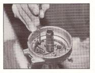
The center-plate slots and the outer ends of the center plate control maximum advance. The stop pins were moved forward to restrict the amount of travel on the center plate. This limits the amount of total advance at the upper rpm range. Too much advance can also be a bad thing.
