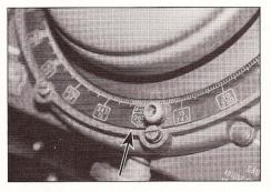
left of zero above the ruled markings at whatever degrees advance the distributor put out at a given rpm.
