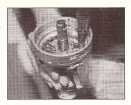
The spring tabs were bent inward to reduce spring tension, allowing the weights to move out with less centrifugal force (lower rpm) and resulting in increased timing advance.
