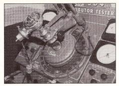
We determined the stock timing advance by testing the distributor on the Sun 504 distributor machine. The stock distributor was spun at 500-rpm increments for comparison with the new, recurved figures.
