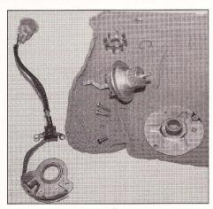
The distributor's stator wheel and pickup coil sender were also removed to gain access to the advance springs and weights below.
