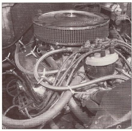
You can economically increase engine performance, whether stock or modified, by changing the advance curve of your distributor. Even a stock engine can produce better throttle response, more low-end torque and better gas mileage.
