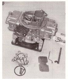
the air horn, the vacuum produced by the pistons of the engine reduces the pressure to about 5 psi, while a pressure of 15 psi (at sea level) acts upon the gasoline in the float bowl. This difference in pressure forces a lot of gasoline from the float bowl into the air passage and into the cylinders, producing the rich mixture necessary to start a cold engine. As soon as the engine is warm, the choke valve must be opened in order to restore the normal air/fuel ratio.
